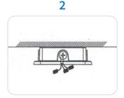
2) Install the junction box to ceiling position.
