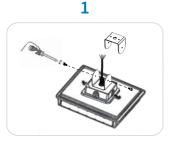
Remove two bolts of the Trunnion Mount and release the Top Trunnion Mount.
