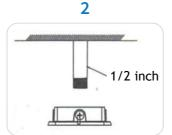
2) Install the junction box to ceiling pendant position.
