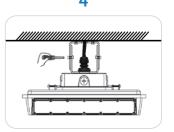
Check that the power line is properly installed and tighten the two bolts of the screw.
