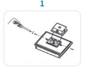
Loosen the two bolts of the LED Junction-box and release the Junction-Box.
