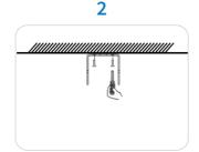
2) Install the Top Trunnion Mount to the ceiling.
