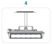
Check that the power line is properly installed and tighten the two bolts of the screw.
