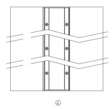
4. Confirm that lamp are worked first, and then disconnect the power, put the lamp into the embedded parts, and then fix the lamp on the embedded box with the inner hexagon cylindrical head machine wire, power on again, finnaly confirm if the lamp are worked again
