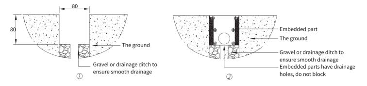
1.Grooves no smaller than the size indicated in the drawing should be reserved at the designated position.There must be a drainage tank or other drainage structure at the bottom of the tank to ensure smooth drainage.
