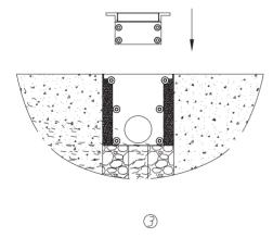
3. Start laying the circuit, connect the blue and brown lights to the negative and positive terminals of the power supply respectively. The connection box of IP68 protection grade is used, and the plug of both male and female IP67 should be wrapped with high pressure waterproof tape. Or take other protective measures up to IP68. After confirming the connection of the lamp, try to switch on the power supply and check whether the lamp lights up normally.
