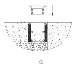
3. Start laying the circuit, connect the blue and brown lights to the negative and positive terminals of the power supply respectively. The connection box of IP68 protection grade is used, and the plug of both male and female IP67 should be wrapped with high pressure waterproof tape. Or take other protective measures up to IP68. After confirming the connection of the lamp, try to switch on the power supply and check whether the lamp lights up normally.
