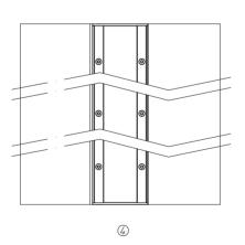
4. Confirm that lamp are worked first, and then disconnect the power, put the lamp into the embedded parts, and then fix the lamp on the embedded box with the inner hexagon cylindrical head machine wire, power on again, finnaly confirm if the lamp are worked again
