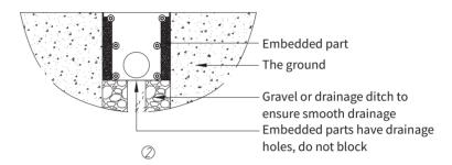
2. Place the embedded parts, connect the wiring pipe, and arrange the corresponding lines (signal lines and power lines). The surrounding of the embedded parts is fixed with cement mortar. If the surrounding areas are flat and firm, screws can be selected to fix according to the actual situation
