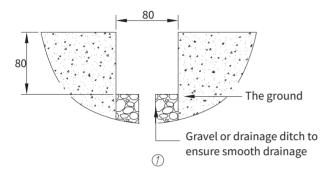
1. Grooves no smaller than the size indicated in the drawing should be reserved at the designated position. There must be a drainage tank or other drainage structure at the bottom of the tank to ensure smooth drainage.
